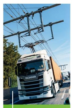
SINCE 2020, OUR 44-TON CATENARY HYBRID TRUCK EL FONDO BY SCANIA HAS BEEN TRAVELLING THE OVERHEAD TEST SECTION OF THE A5 AUTOBAHN.
